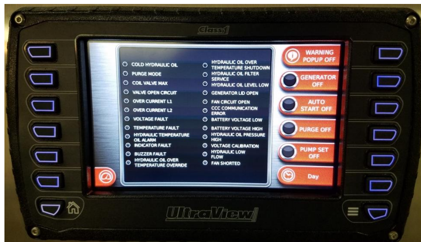
Figure 26 – J1939 Multiplex Control and Diagnostic Information
