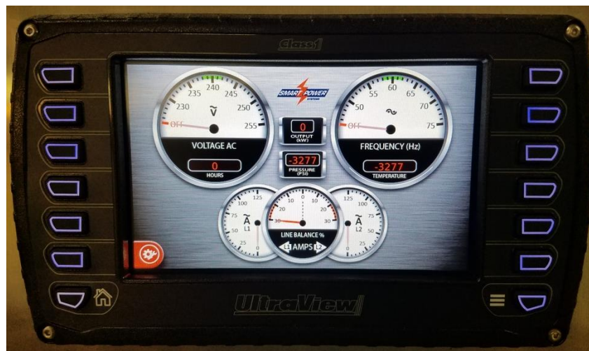
Figure 25 – J1939 Multiplex Monitoring
