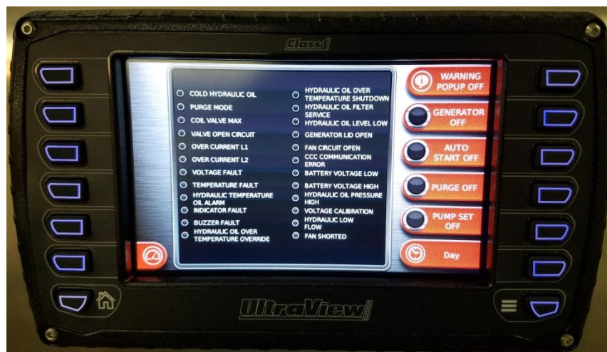
Figure 26 – J1939 Multiplex Control and Diagnostic Information
